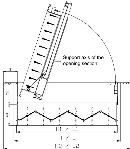
WS-101-D-A-F – SECTIONS WITH DAMPER
