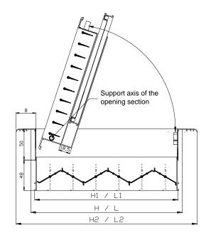
WS-101-D-A-F - SECTIONS WITH DAMPER
